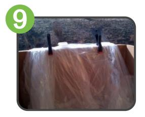
As the bag empties inside of the tote, pull up the bag and clamp it to the edge to allow oil to drain down towards the lower drain fitting.
