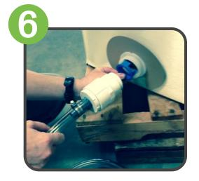
Unscrew the plug found in the lower drain fitting of the tote. Inside, you will find a cutter. Pull this cutter out and flip it around so that the sharp teeth are facing in. Reinsert it into the lower drain fitting with the teeth facing towards the tote.
