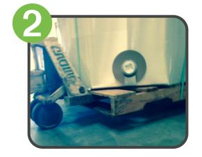
To use this tote dispensing attachment, you'll want to elevate the tote to allow the oil to gravity feed out. One common way to do this is to store your pallet on a pallet rack or shelf. Another is to elevate it a few inches off of the ground. To complete this, first lift the pallet up using a pallet jack or fork lift.
