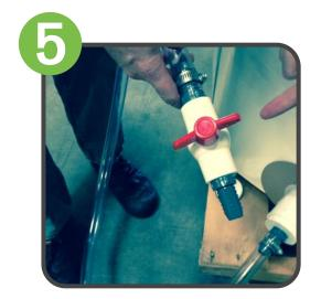
You will now connect the dispensing attachment. Before beginning this process, it's very important to make sure that the valve is in the closed position (as shown) with the colored valve perpendicular to the hose.
