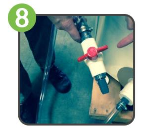
As you screw the fitting in, the cutter will pierce the tote bag and oil will begin running into the clear tubing. Once the attachment is all screwed in, simply turn the valve and oil will begin to flow into your desired container.
